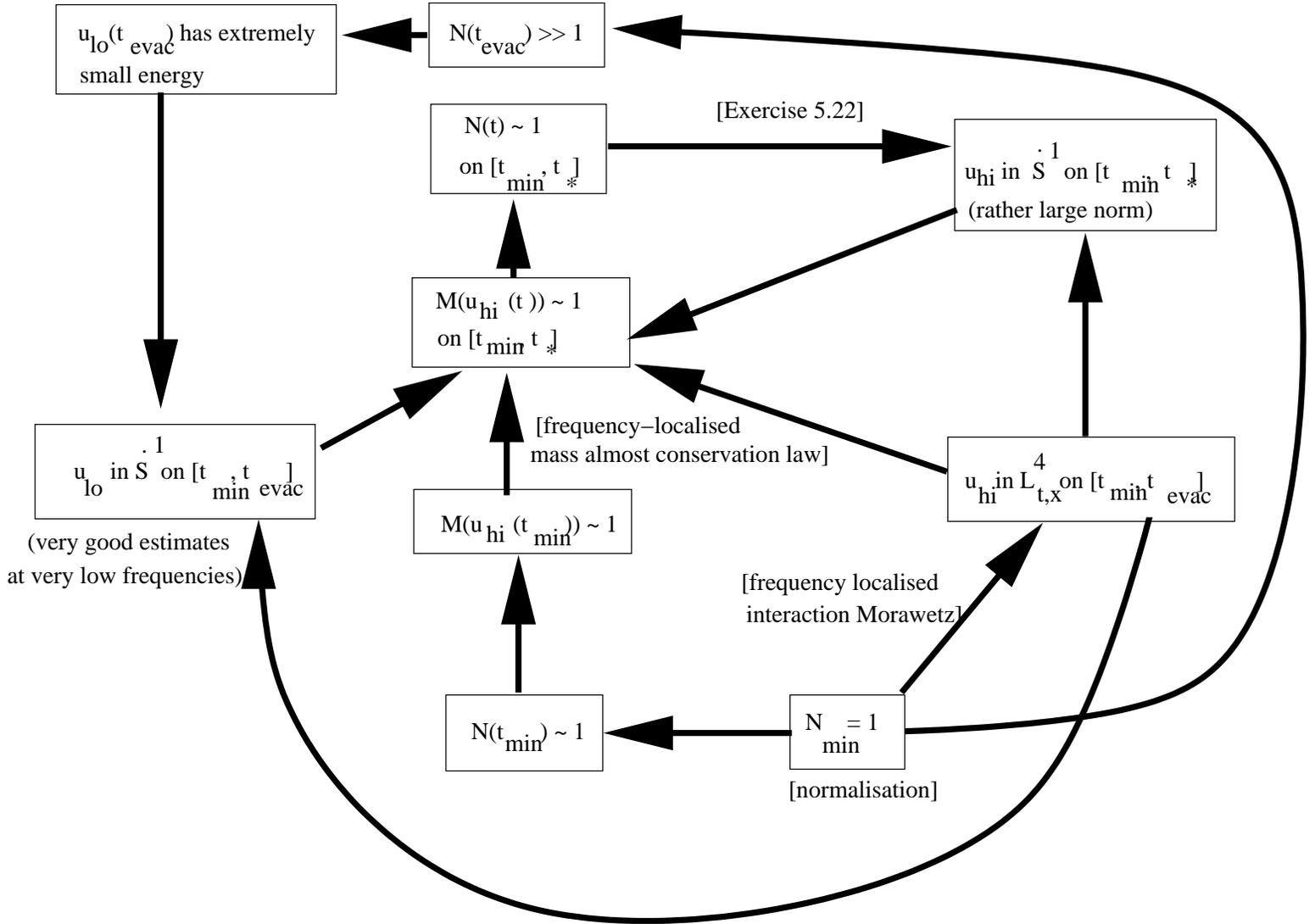
FIGURE 14. A schematic depiction of the global mass almost conservation law. A continuity argument allows one to push  $t_*$  up to  $t_{evac}$ , obtaining the contradiction.
