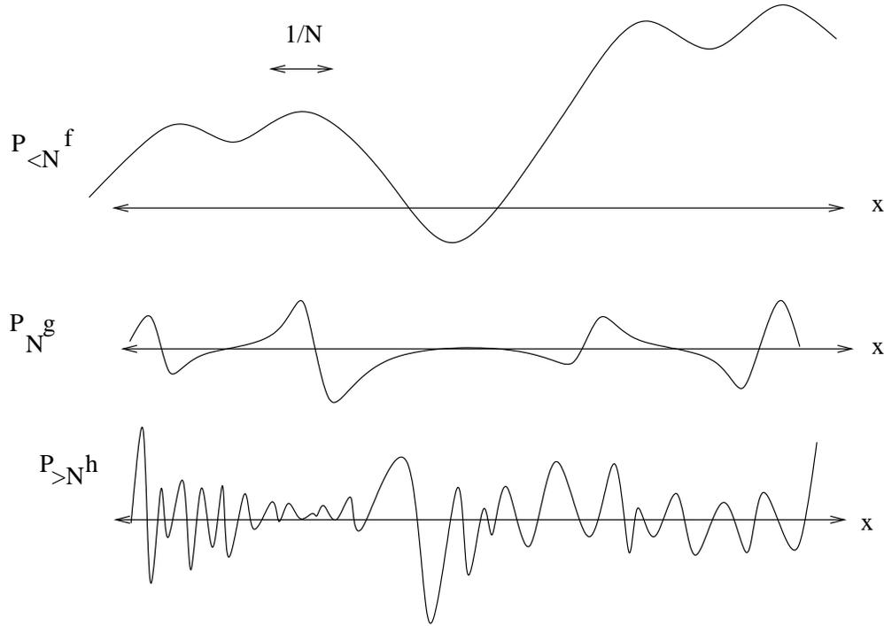
FIGURE 1. The uncertainty principle. The low-frequency function  $P_{<N}f$  has frequencies less than  $N$  and is thus essentially constant at spatial scales  $\ll 1/N$ . The high-frequency function  $P_{>N}h$  has frequencies greater than  $N$  and thus oscillates (with mean essentially zero) at spatial scales  $\gg 1/N$ . The medium-frequency function  $P_Ng$  behaves in both fashions simultaneously.
