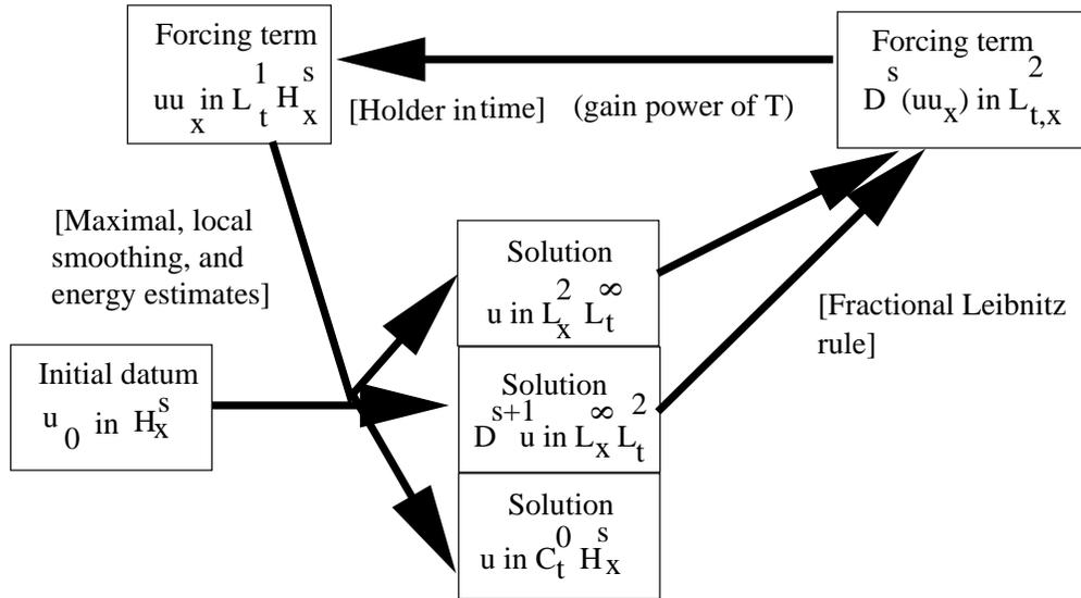
FIGURE 1. Iteration scheme for KdV using local smoothing and maximal function estimates. Note the interchange of time and space integration at various locations in the scheme. The situation for mKdV is similar, but with  $u$  in  $L_x^4 L_t^\infty$  rather than  $L_x^2 L_t^\infty$ , and with a nonlinearity of  $u^2 u_x$  rather than  $uu_x$ .
