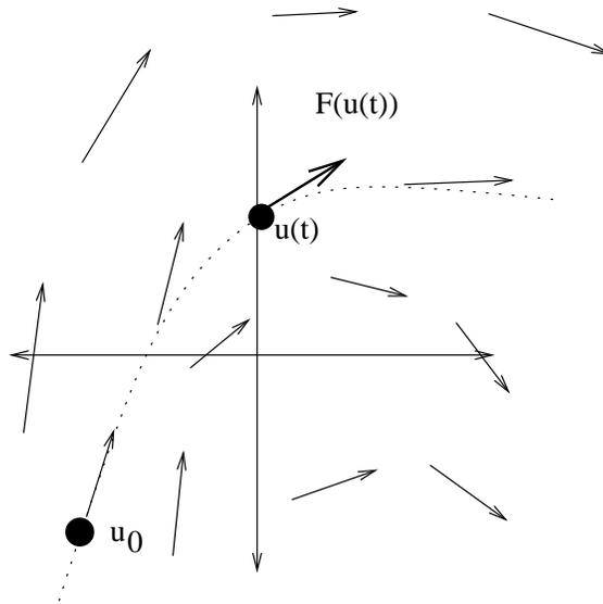
FIGURE 1. Depicting  $F$  as a vector field on  $\mathcal{D}$ , the trajectory of the solution  $u(t)$  to the first order ODE (1.7) thus “follows the arrows” and *integrates* the vector field  $F$ . Contrast this interpretation of an ODE with the rather different interpretation in Figure 2.
