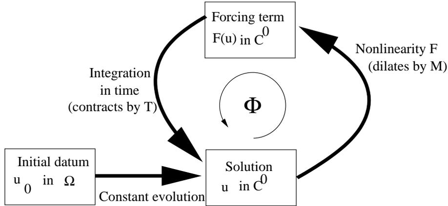
FIGURE 3. The Picard iteration scheme. The map  $\Phi$  is basically the loop from the solution  $u$  to itself. To obtain the fixed point, start with the initial datum  $u_0$  as the first approximant to  $u$ , and apply  $\Phi$  repeatedly to obtain further approximations to  $u$ . As long as the net contraction factor  $T \times M$  is less than 1, the iteration scheme will converge to an actual solution.
