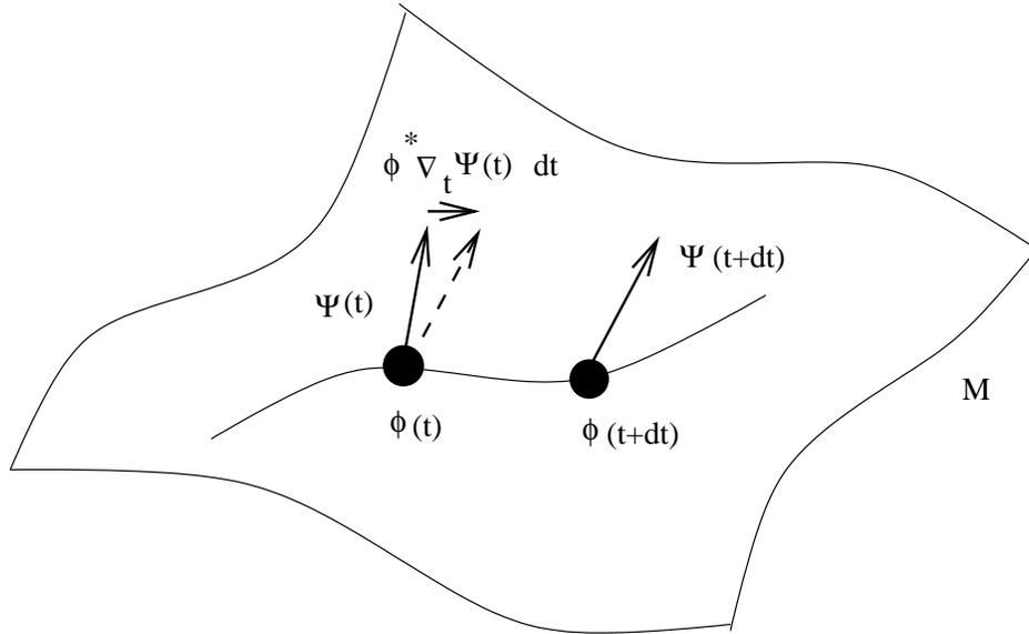
FIGURE 1. An infinitesimal viewpoint of the covariant derivative. One uses parallel transport to bring the tangent vector  $\Psi(t + dt)$  from  $T_{\phi(t+dt)}M$  to  $T_{\phi(t)}M$ , where it is then compared against  $\Psi(t)$ .
