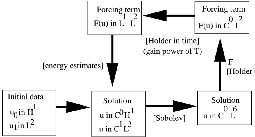
FIGURE 6. A simple iteration scheme in  $H_x^1 \times L_x^2$ , based on the energy estimate, for the three-dimensional cubic NLW  $d = 3, p = 3$ . For higher powers  $p$ , Strichartz estimates and spaces are needed.
