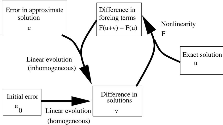
FIGURE 10. The difference scheme for an approximate perturbation  $\tilde{u} = u + v$  to an exact solution  $u$ . This scheme can also be reversed to convert an approximate solution  $\tilde{u}$  to an exact solution  $u = \tilde{u} - v$  (by replacing  $F(u + v) - F(u)$  with  $F(\tilde{u}) - F(\tilde{u} - v)$ ).
